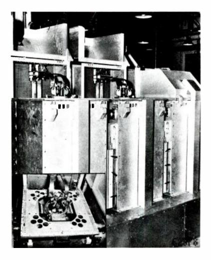
Driver and Final Amplifier Tanks. Insert is a top view showing the Type 5592 tube used in these stages.
